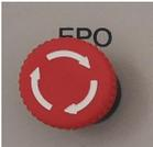
Clockwise rotate before load bank operation
