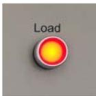
4) Push on the "Load"--Main contactor on, loading activated
