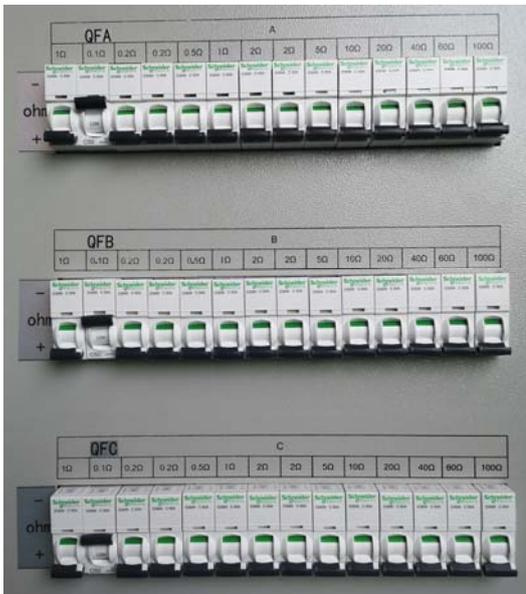
5) Make sure **ALL** circuit breakers are OFF, then push on QFA(0.1ohm), QFB(0.1ohm), QFC(0.1ohm) circuit breakers--load bank **ALL** resistors are loading (see above picture & below diagram)
