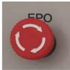
1) Clockwise rotate before load bank operation
